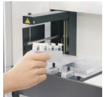
Fig. 6. Large reagent vial rack for unattended runs
