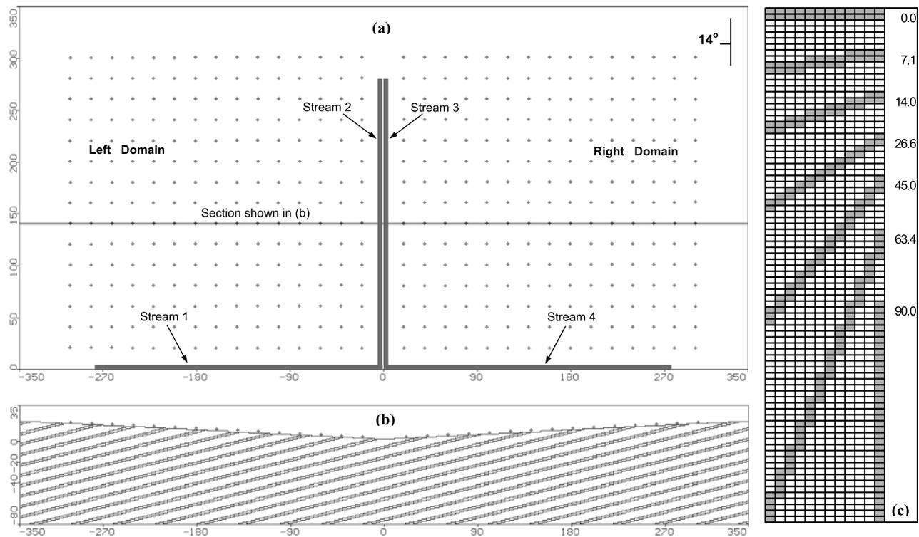
**Figure 4.** (a) Model plan view, showing the streams (numbered 1–4) and the 225 particles placed in each domain, (b) model cross-section view showing dipping beds, and (c) representation of dipping beds in MODFLOW at various dip angles.
