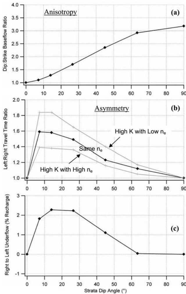
**Figure 9.** Effect of strata dip angle: (a) dip:strike ratio in base flow, a measure of flow anisotropy, (b) left:right ratio in particle travel time, a measure of flow asymmetry, and (c) groundwater flow under the central streams from the right to the left domain, as percent recharge.
