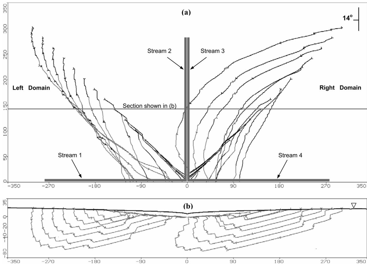
**Figure 6.** Simulated flow pathways for a more permeable weathered zone, projected to (a) plan view and (b) cross-section view. Black segments are going into and gray segments are coming out of the page. Each tick mark on the path lines indicates 10 years of travel time.
