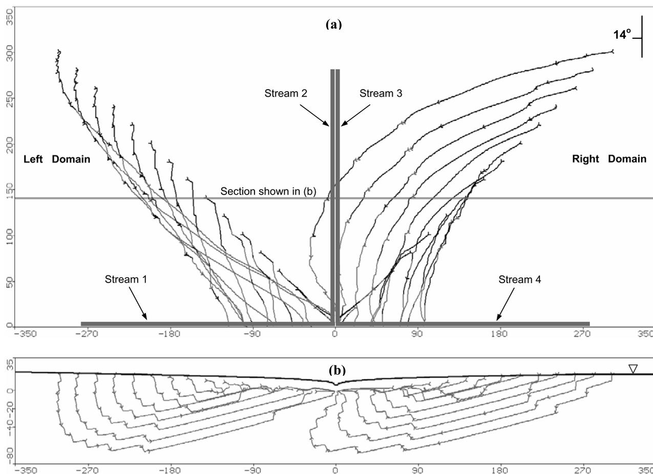
**Figure 5.** Simulated flow pathways for the base case, projected to (a) plan view and (b) cross-section view. Black segments are going into and gray segments are coming out of the page. Each tick mark on the pathlines indicates 10 years of travel time.
