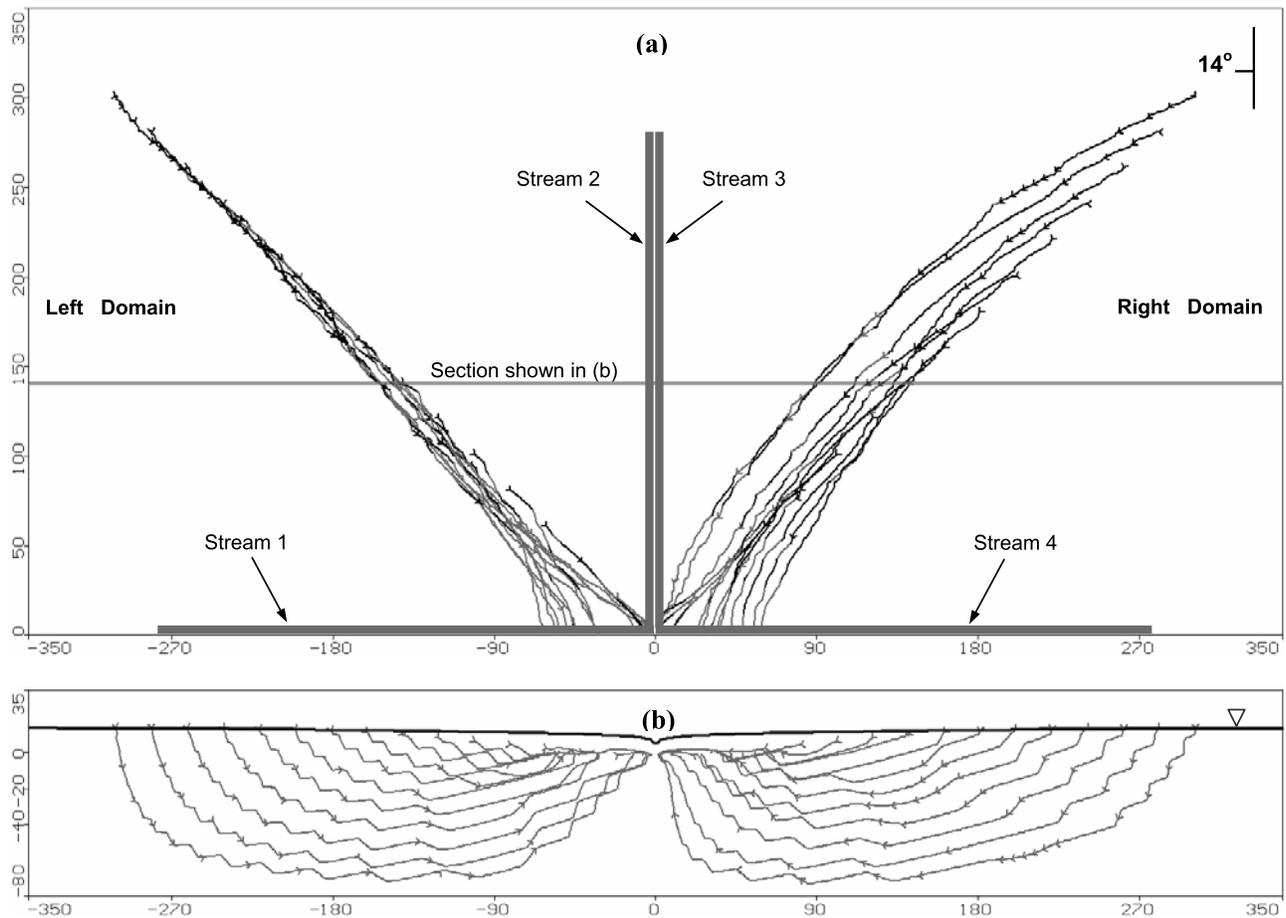
**Figure 7.** Simulated flow pathways for weaker bedding anisotropy, projected to (a) plan view and (b) cross-section view. Black segments are going into and gray segments are coming out of the page. Each tick mark on the path lines indicates 10 years of travel time.
